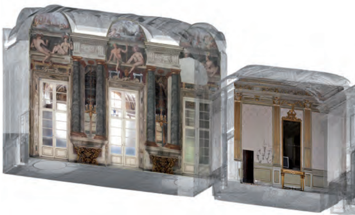
Fig. 35 - Digital survey of the rooms on the main floor: digital processing of the 3D point cloud, with insertion of photo planes on the walls and vaults
