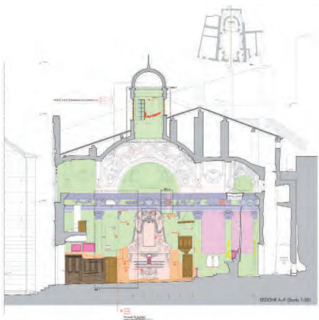
Fig. 83 - Map of the materials: longitudinal section a-a'
