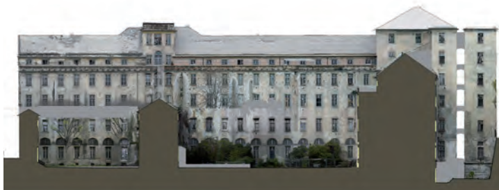
Fig. 40 - Reinstatement of the photogrammetric survey: east-west transversal section of the entire complex of the Albergo dei Poveri with insertion of orto-photos
