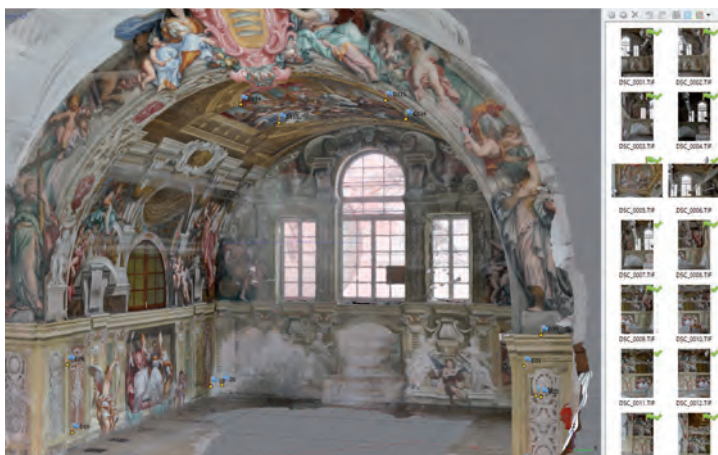
Fig. 25 - Three-dimensional model of the barrel vault of the reading room obtained using Structure From Motion
