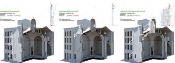
Fig. 84 - Three-dimensional model: possible local mechanisms of collapse
