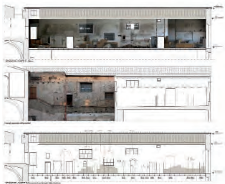
Fig. 118 - Survey and interpretation of the characteristic elements and the stratigraphic evidence
