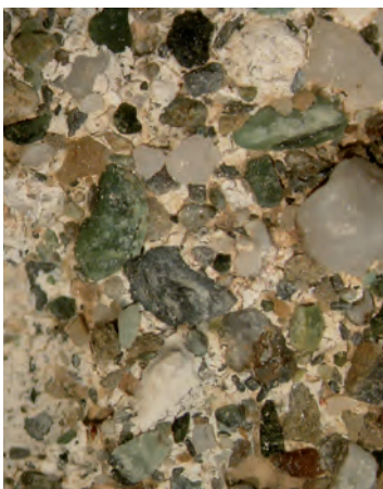
Fig. 12 - Plaster taken from vico Croce Bianca 10 containing sand from Sampierdarena, used between the XV and XIX centuries
