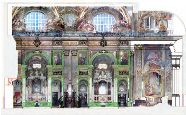
Fig. 205 - Longimetric survey of the longitudinal section with the insertion of photo planes
