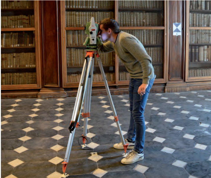
Fig. 9 - Topographical relief with Total Station. Former Library of the Jesuit College
