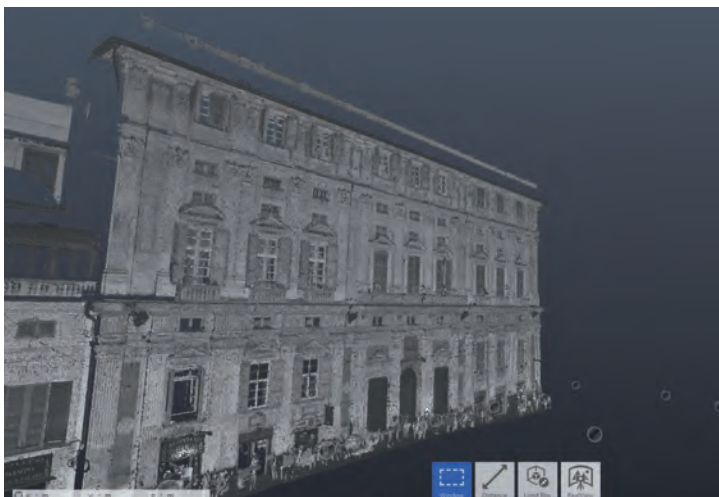
Fig. 3 - View of the point cloud obtained by laser scanner survey. Palazzo Belimbau, facade overlooking Piazza della Nunziata, Genoa
