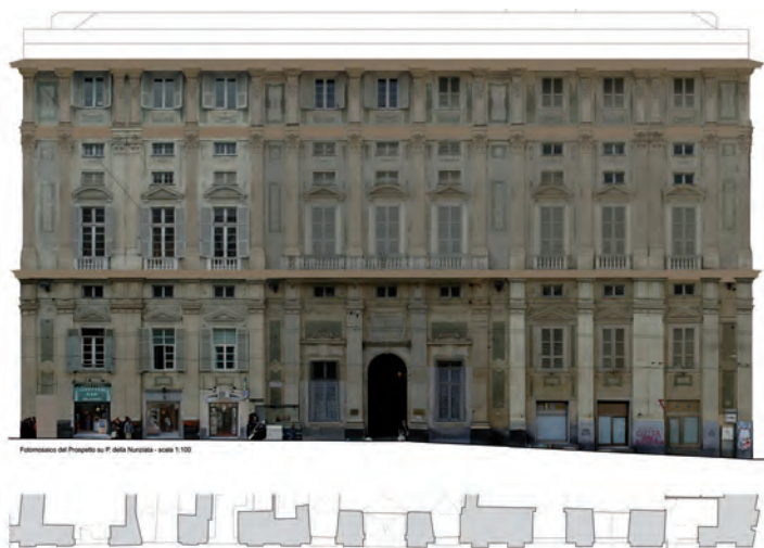
Fig. 34 - Digital relief: photographic straightening of the principal facade
