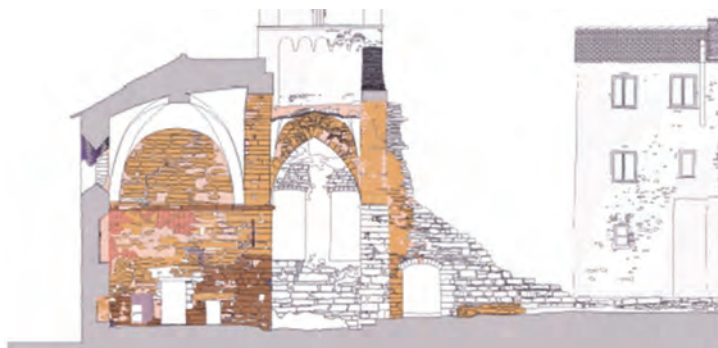
Fig. 247 - Map of the degradation phenomena
