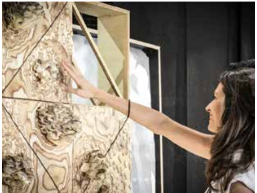
◀ IAAC – IAAC-CFC, “Myco-Scape”, 2019, a modular system which supports the growth of edible mushrooms in the urban environment (public space/facades/rooftops), producing both food and construction materials.
