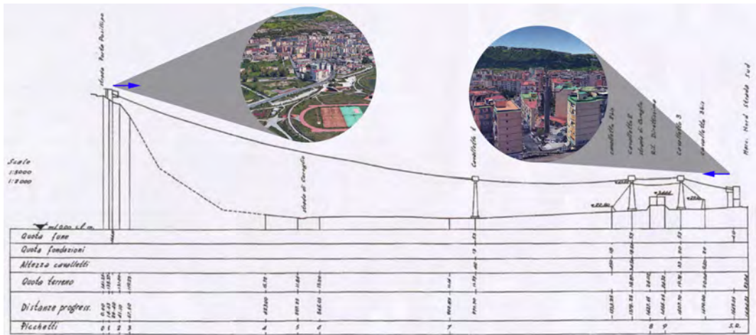
Fig.9 Graphic of the altimetric route of the ropeway (Source: Archive of the Mostra D'Oltremare, 1952) with images of today's “moving panorama”.
