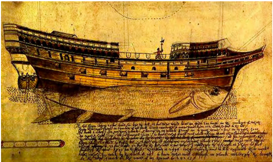
Fig. 4 The hull of a vessel inspired by the shape of a cod head and a mackerel tail. Matthew Baker, Fragment of Early English Shipwrihty (1586), Magdalene College, Pepys Library, Cambridge (Ms 2820, sheet n.d.).
