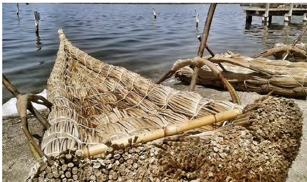
Fig. 5 Cabras ponds, Sinis (Sardinia). Fassonis on the shore, view of the binding systems and the forward closure.
