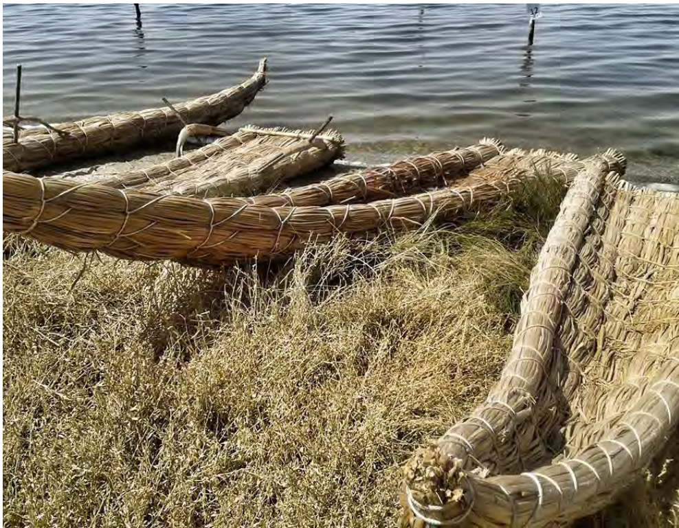
Fig. 4 Cabras ponds, Sinis (Sardinia). Fassonis on the shore, aft view on the assembly systems of the bundles.
