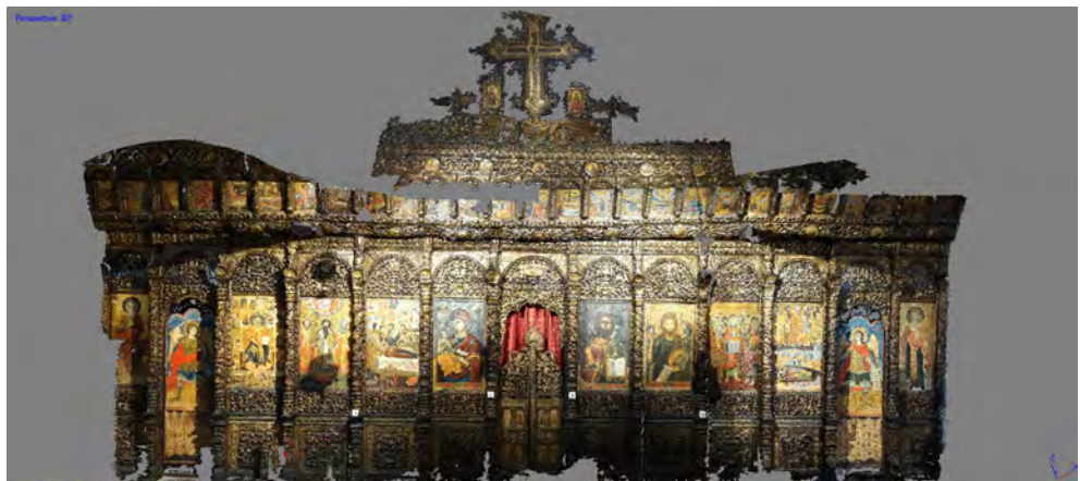
Fig. 11 Albania, Berat, Onufri Museum, altar; indirect digital photogrammetric relief. Modeling software with image superimposition, point clouds and mesh detection
