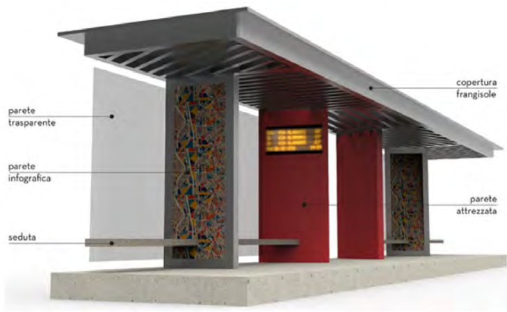
Fig. 8 The elements of a standard canopy
