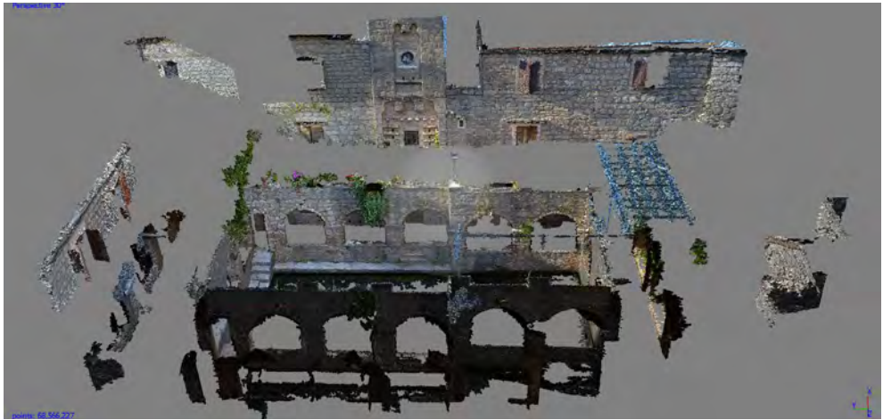
Fig. 2 The Fortress of Hvar Tvrđalj, cloud of the points of the inner courtyard, the fish tank and the vaulted system
