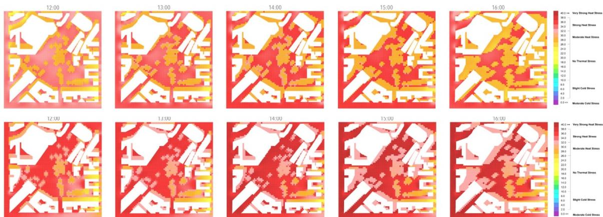
Figure 4. Simulation results – UTCI mapping for July 30<sup>th</sup> (above) and July 18<sup>th</sup> (below).
