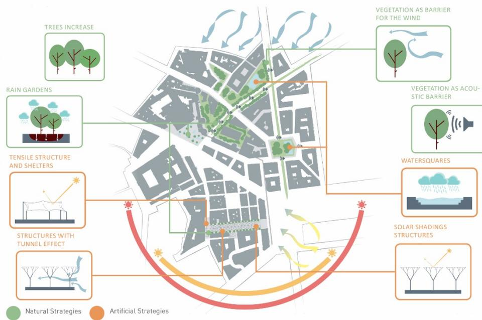
Figure 6. Synthesis of the main adaptive design strategies applied in the project.
