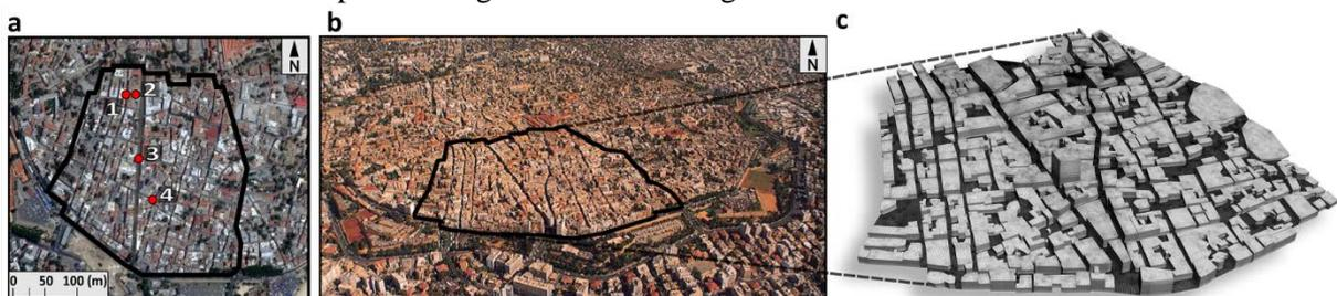
Figure 1. (a) Top view and (b) aerial view of the case study. (c) high-resolution computational grid on the building surfaces (14,670,517 hexahedral cells).
